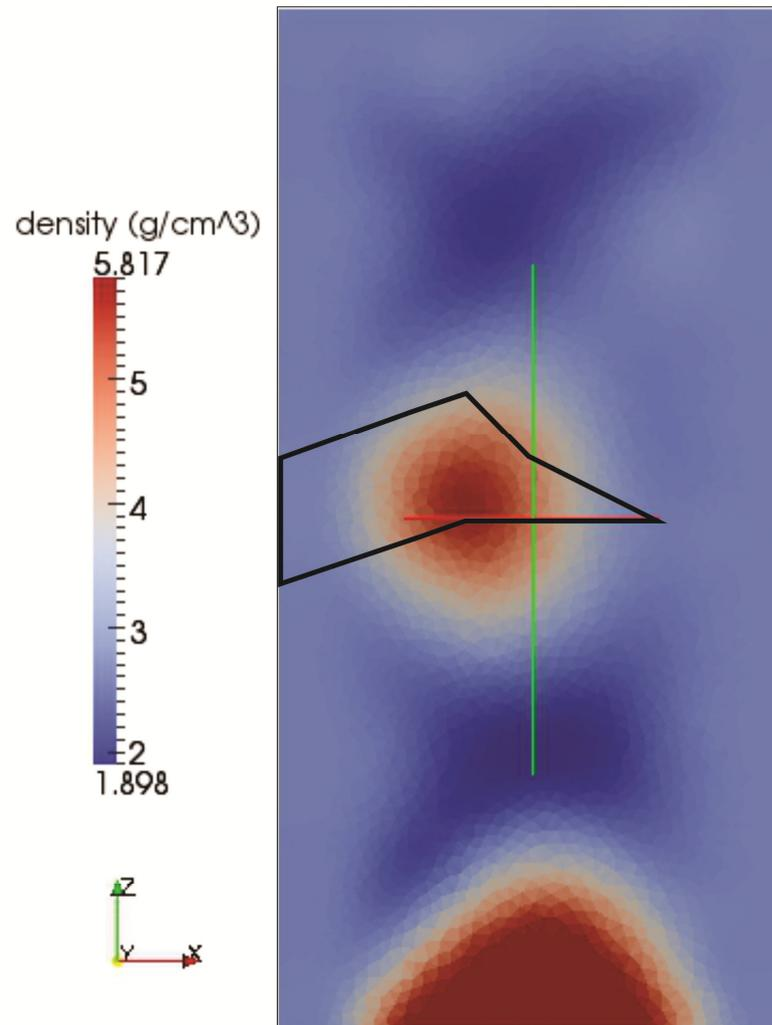
Gravity-only inversion of moderate noise data from borehole A and B stations
