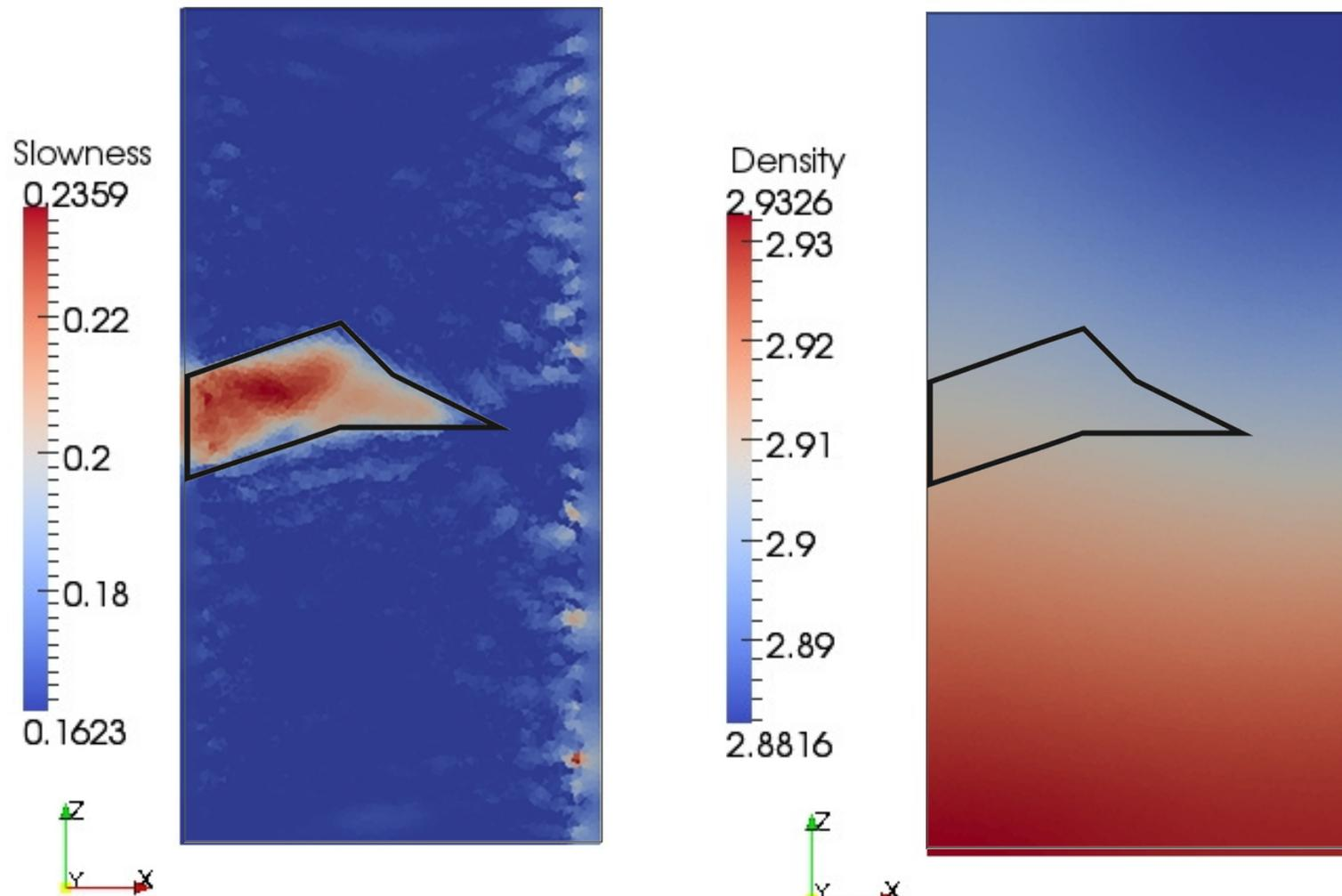
Joint Inversion of high noise data using a low similarity parameter, gravity data from surface stations only
