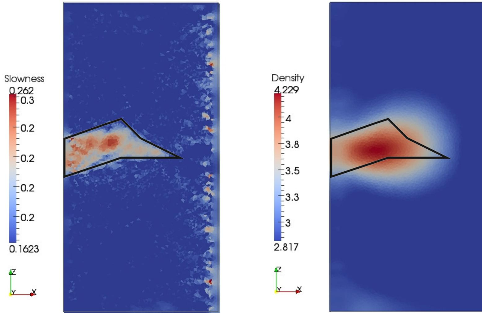
Joint inversion of moderate noise data, gravity data from borehole B data
