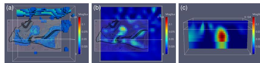
Figure 4 : Magnetic susceptibility model (SI) from independent inversion with default depth weighting: (a) top view of 0.025 threshold, (b) and (c) as for Fig. 3.
