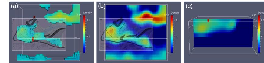
Figure 11 : Density model (g/cc) from cooperative inversion: (a) top view of 0.07 threshold, (b) and (c) as for Fig. 3.
