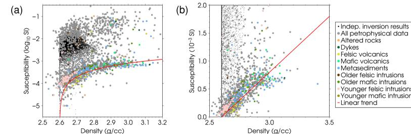
Figure 7 : Petrophysical information available for the Kristineberg area (various colours), all petrophysical information for the Skellefte district (grey), and recovered model values from the independent inversions (black). The red line shows the linear trend used in the joint inversion with petrophysical coupling (Fig. 9). Panel (a) has  $\log_{10}$  scale for susceptibility whereas panel (b) has linear scale and only shows a portion of the full range of data.
