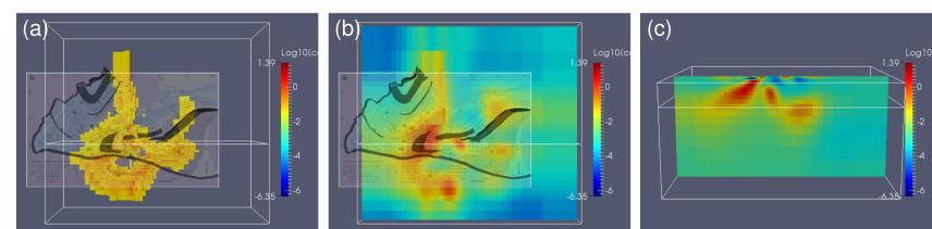
Figure 6 : Conductivity model ( $\log_{10}$  S/m) from independent inversion, from the work of [6]: (a) top view of -1.5 threshold, (b) and (c) as for Fig. 3.
