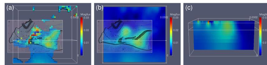
Figure 5 : Magnetic susceptibility model (SI) from independent inversion with reduced depth weighting: (a) top view of 0.007 threshold, (b) and (c) as for Fig. 3.
