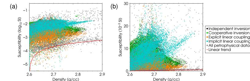
Figure 8 : Density versus susceptibility scatter plots for models recovered from various inversions. The red line shows the linear trend used in the joint inversion with petrophysical coupling (Fig. 9). Panel (a) has  $\log_{10}$  scale for susceptibility whereas panel (b) has linear scale. The vertical axes in both panels do not cover all recovered values: some of the lowest susceptibility values are not plotted in (a) and some of the highest values are not plotted in (b).
