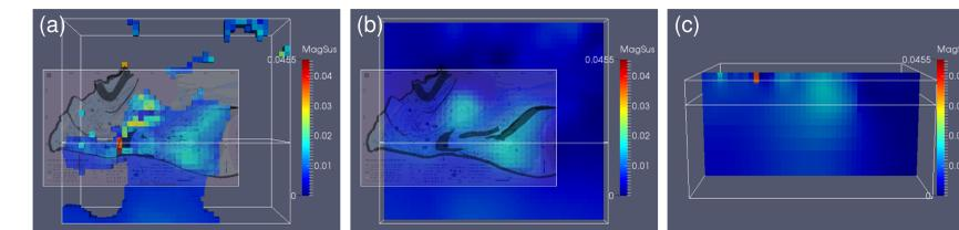
Figure 12 : Magnetic susceptibility model (SI) from cooperative inversion with reduced depth weighting: (a) top view of 0.007 threshold, (b) and (c) as for Fig. 3.
