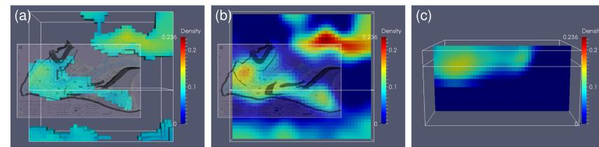
Figure 3 : Density model (g/cc) from independent inversion: (a) top view of 0.07 threshold, (b) top view of -4km depth slice, (c) side view looking north of northing = 20km slice. Panels (a) and (b) include opaque interpreted surfaces (black) and geological map.
