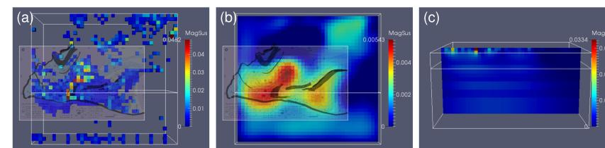
Figure 9 : Magnetic susceptibility model (SI) from joint inversion with explicit linear coupling and reduced depth weighting: (a) top view of 0.005 threshold, (b) and (c) as for Fig. 3. The upper colour-scale limits in (b) and (c) have been changed to accentuate the recovered features.
