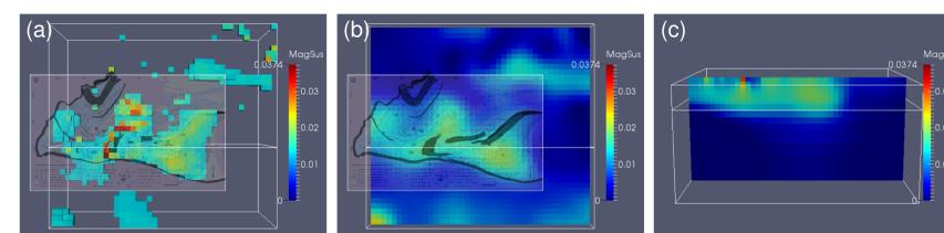
Figure 10 : Magnetic susceptibility model (SI) from joint inversion with implicit linear coupling and reduced depth weighting: (a) top view of 0.0125 threshold, (b) and (c) as for Fig. 3.
