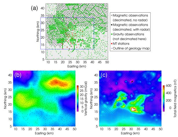
Figure 2 : (a) Data observation locations, (b) gravity response after regional removal (decimated here), (c) magnetic response after regional removal. Coordinates are in our own system.
