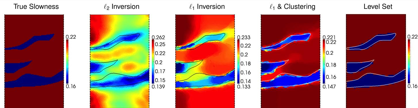
True and recovered models for a cross-well tomography example. The outlines of the true bodies are superimposed in black or white on top of the recovered models. Lines of down-hole sources and receivers are displayed as black dots. The colour-bars show slowness in s/km. The meshes are 60 m by 100 m.
