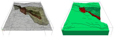
55x82x31=139,810 cells and stair-casing still evident
